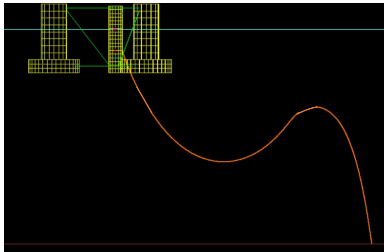
Figure 2-6: OrcaFlex model of the steep wave dynamic power cable configuration
