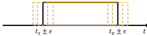
Figure 6.3: Relaxed Data Augmentation. t_s^g and t_e^g refer to the start and end of action in the ground truth whereas \epsilon denotes the \pm 2 frames i.e, \epsilon \in \{-2 \times \frac{1}{15}, -1 \times \frac{1}{15}, 0 \times \frac{1}{15}, 1 \times \frac{1}{15}, 2 \times \frac{1}{15}\} seconds relaxation for augmentation.
