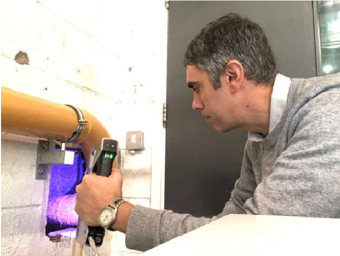
Figure 41: Undefined hole in the building envelope. Figure 42: Manual 3D scanning of hole
