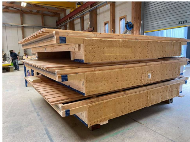
Figure 39: Wood fibre strip 20-30mm thick Figure 40: MAKAR timber panels with wood fibre strip between panels
