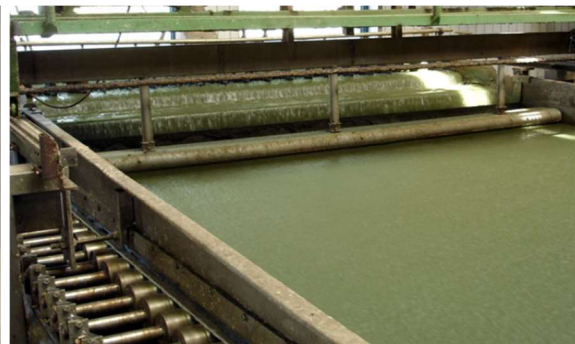
Figure 3: Wood-water mix is delivered into a mould
