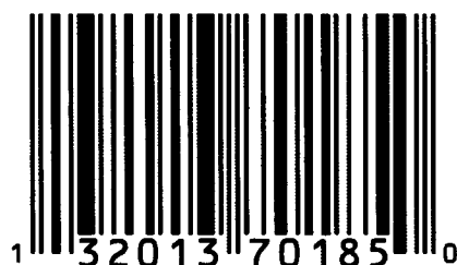
Figure 6.1 Example of a UPC standardised product barcode. A series of 12 digits and an associated series of bars and spaces coding for the same numbers
