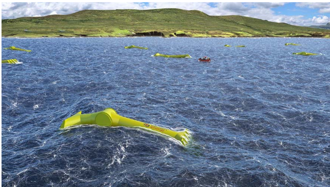
Figure 4.1. Illustration of an array of eight Blue Horizon 1 MW-scale WECs, from Mocean Energy.
