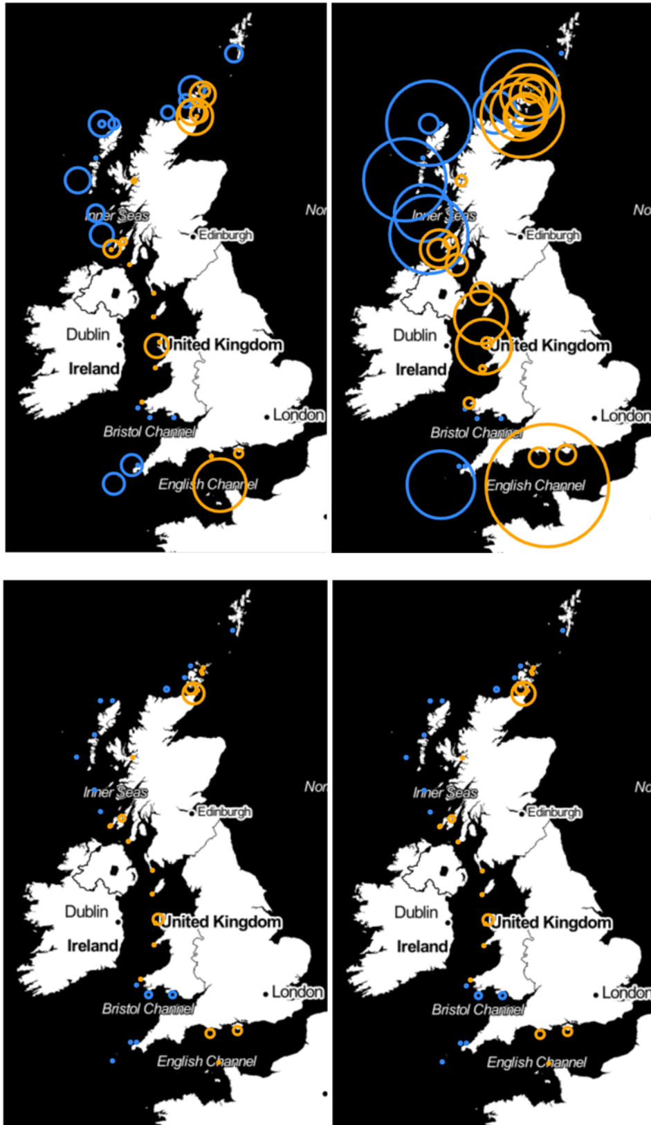
Figure 8.11. Visual comparison of the installed capacities of wave power (blue) and tidal stream (orange) between 'Low Marine' (top left), 'High Marine' (top right), CT (bottom left), LW (bottom right). There is only a very slight difference between CT and LW. Installed capacity is indicated by the area of the bubble.
