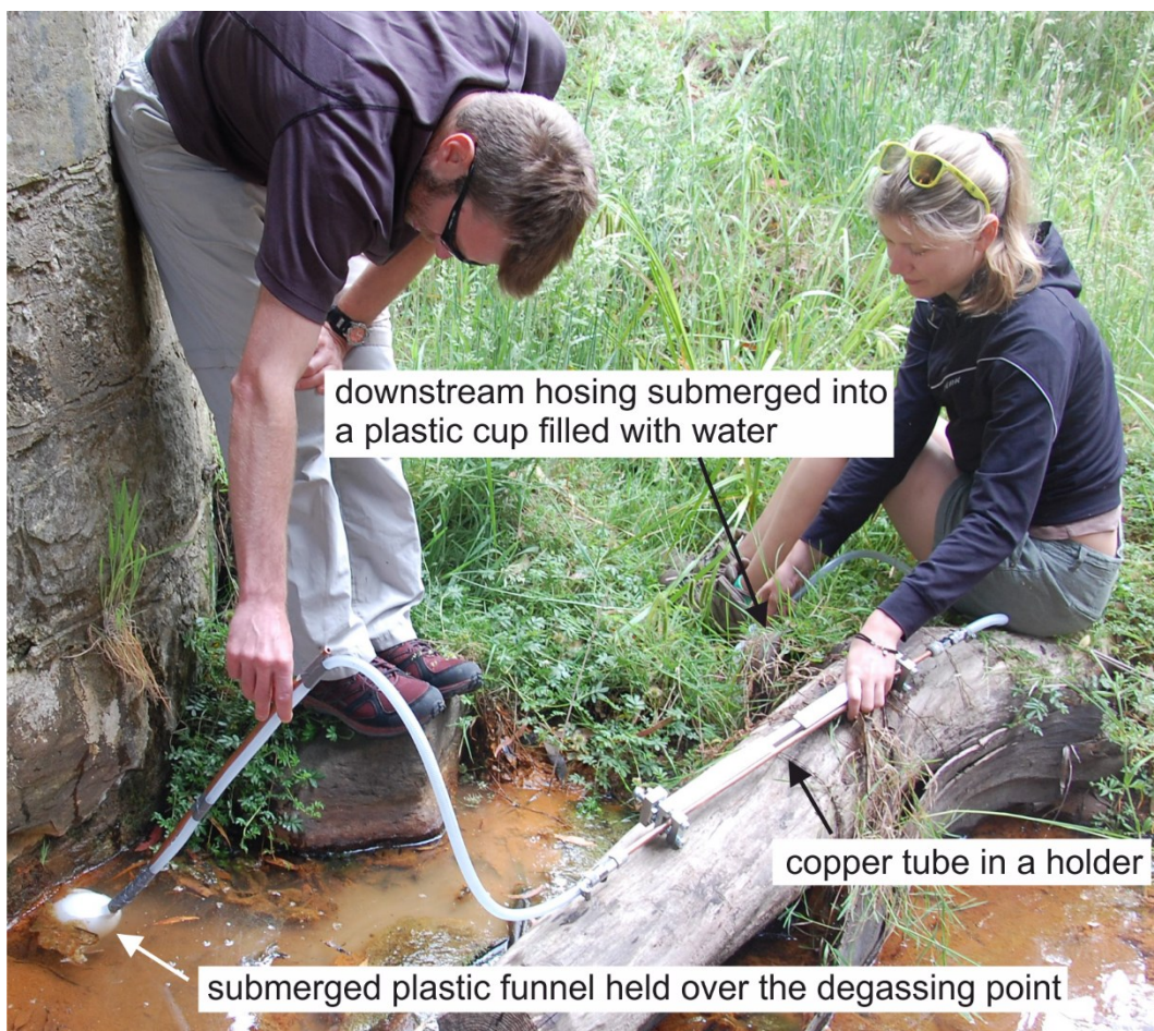
Figure 2.2. Sampling gases from the mineral springs, using the previously described copper tube method. Plastic funnel is submerged under water over the degassing location. The downstream end of the hosing is held submerged in a cup of water to prevent air backflow and monitor the flow rate.
