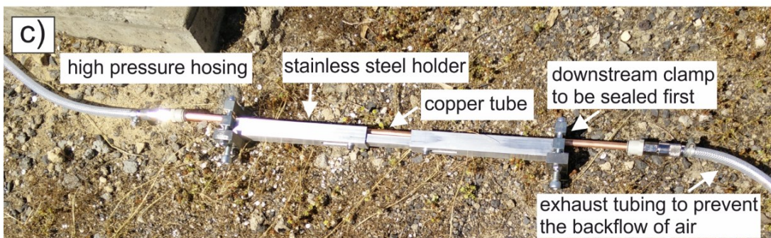
Figure 2.1. Sampling of high pressure gases from the wellhead. b) Close up showing the wellhead sampling port and the step-down pressure regulator. c) Copper tube in a stainless steel holder and two stainless steel clamps attached at both end, with high pressure hosing connecting to the regulator and at the downstream end to prevent the backflow of air.
