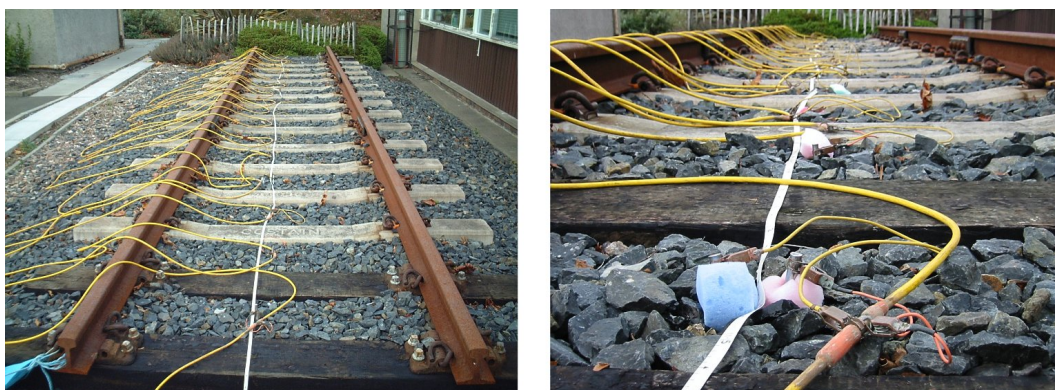
Figure C-4. Photographs of the electrode lay out (left) and the electrodes with the sponges saturated with an electrolyte solution to address the high contact resistance (right)
