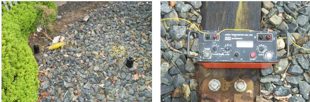
Figure C-7. Photographs of the porous pots (left) and the ABEM Terrameter 300 digital high-input-impedance voltmeter (right)
