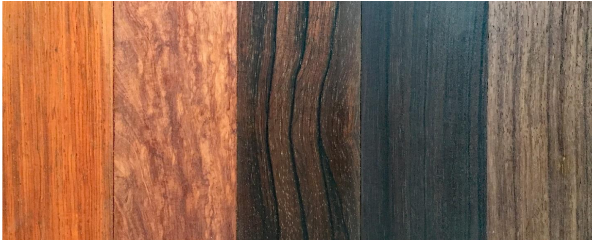
Figure 5.12: Photos of commonly available rosewood species. Depicted from left to right are Cocobolo ( Dalbergia retusa ), Honduran rosewood ( Dalbergia stevensonii ), Brazilian rosewood ( Dalbergia nigra ), African blackwood ( Dalbergia melanoxylon ), and East Indian rosewood ( Dalbergia latifolia ).
