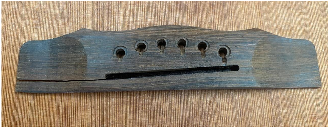
Figure 6.2: Photo of a cracked bridge due to wood failure at the saddle slot. Photo by the author.
