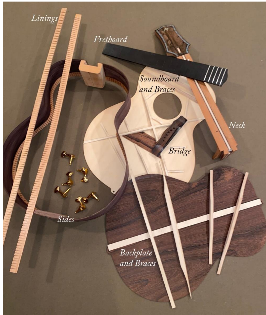
Figure 2.2. Deconstructed view of the components that make up a typical steel-string guitar. Photo by author.
