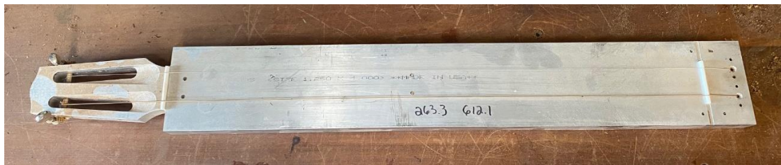
Figure 2.4: A photo of a solid bar-stock aluminum string rig. Because the bar-stock is so stiff, its mechanical resonances are sufficiently high in frequency to effect relatively little influence upon the vibration of the string in the frequency range of interest to human listeners, and subsequent sound radiation characteristics. Hence, the string is essentially “isolated”, allowing for analysis of it in a largely de-coupled state. Photo by author.
