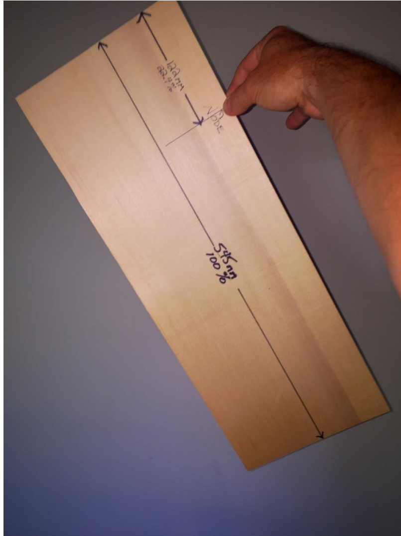
Figure 2.10: A photo demonstrating the technique to hold a tonewood plate at a node to test the tap-tone in the longitudinal direction.
