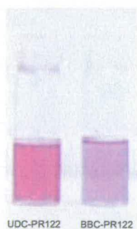
Figure 3.35: Difference of dispersibility between 10-Undecenoyl-modified PR122 (UDC-PR122) and 4-Bromobenzoyl-modified PR122 (BBC-PR122) after 4 days
