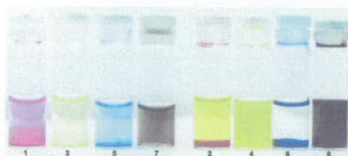
Figure 3.26: Dispersibility of cross-linked compounds in water for (1, 3, 5, 7) and DMF for (2, 4, 6, 8) (1 mg/mL) after 2 weeks
