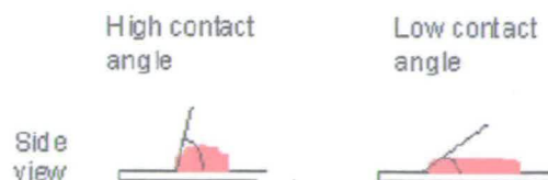
Figure 4.10: Schematic representation of contact angle measurement
