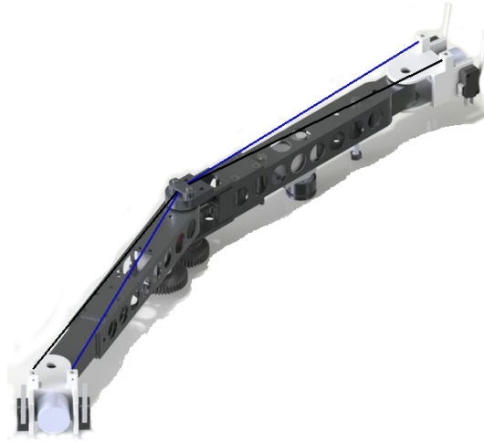
Figure D.2: Depiction of the passive string mechanism, devised to ensure surface alignment at surface contact.
