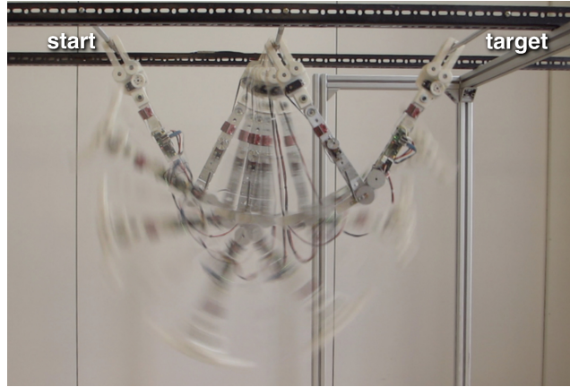
(a) Optimised movement of the robot (single phase locomotion)
