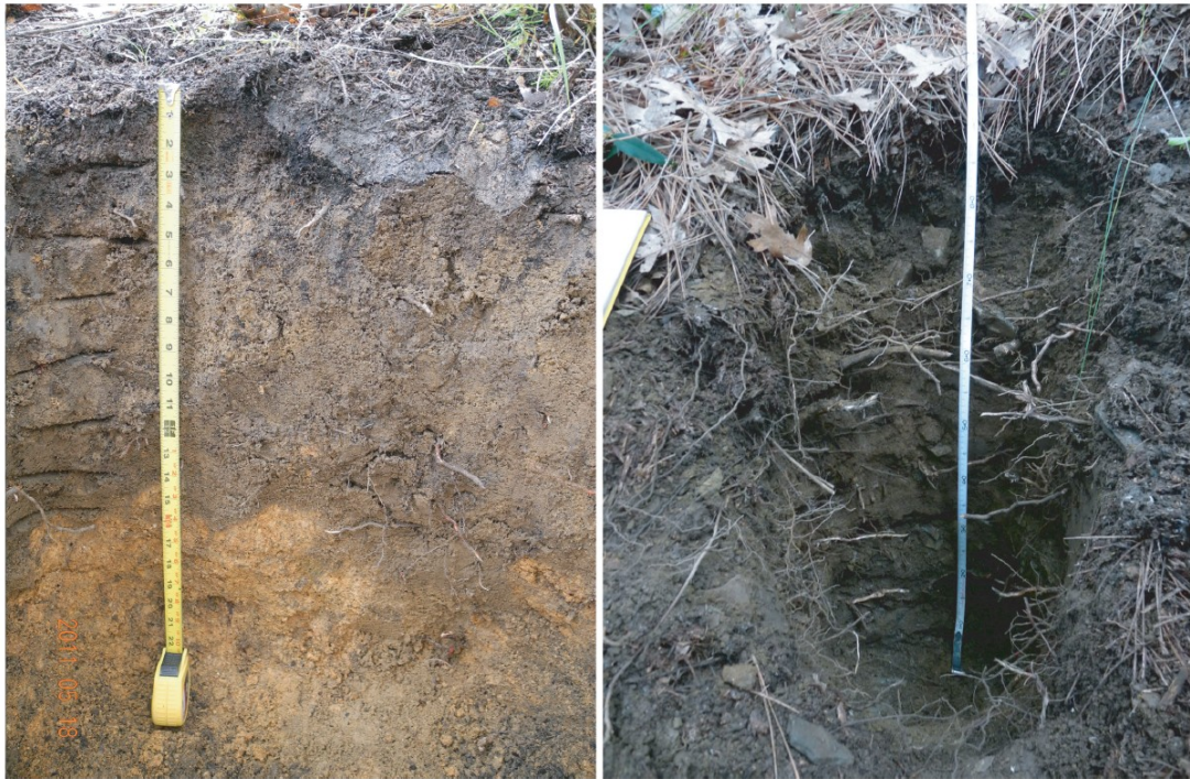
Figure 3.5: Example soil profiles in (a) granodiorite and (b) metavolcanics. Pit in granodiorite comes from hilltop along cascade ridge (red line in Figure 3.4) with hilltop curvature C_{HT} = -0.062 ; pit depth is 65cm. Pit in metavolcanics on steep slope (c. 40^\circ ), pit depth is 85 cm.
