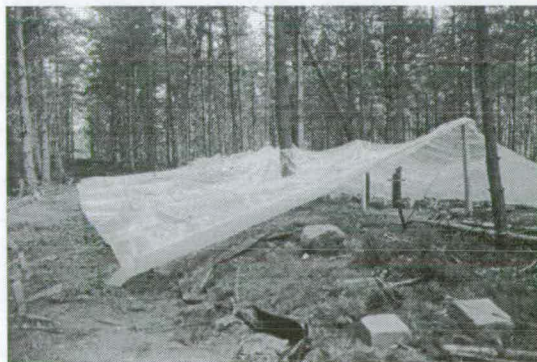
Plate 1. (Left) The experimental plots were isolated from the surrounding soil by a 1.5 m deep ditch, the sides of which were lined in a heavy polythene sheet before being refilled with soil. This prevented lateral inflow of water and allowed the plots to be droughted.
