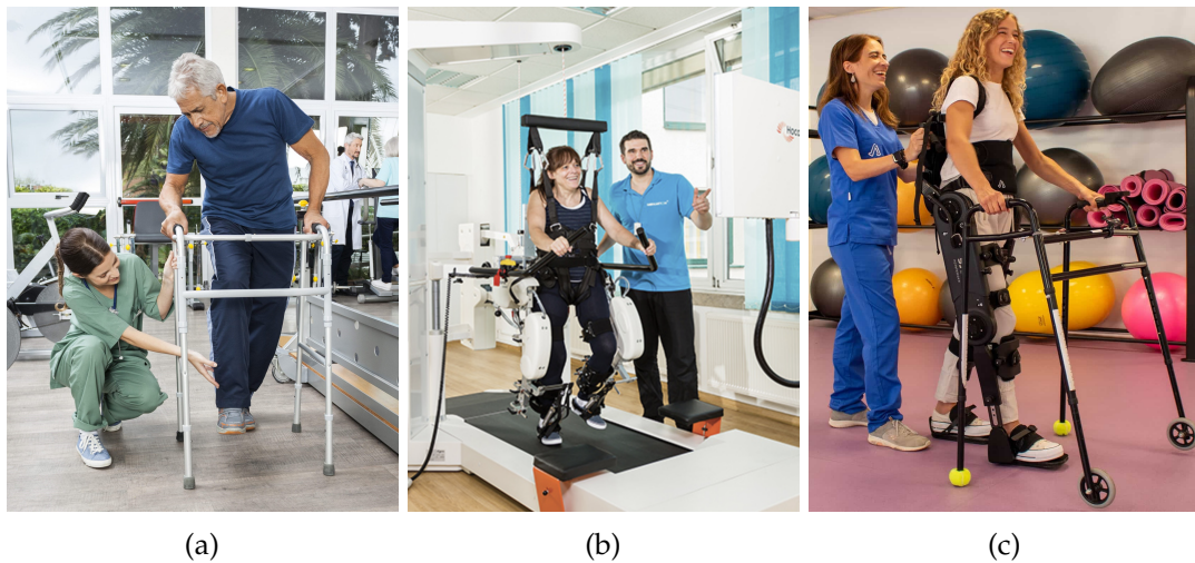
Figure 1: Examples of gait rehabilitation using (a) a walking frame (extracted from [40]), (b) the stationary robotic platform LOKOMAT (extracted from [41]) and (c) the exoskeleton ABLE with a walker (extracted from [42]).
