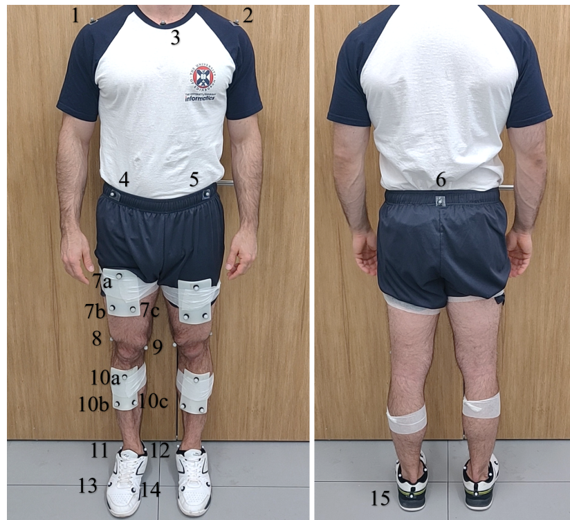
Figure 6: Placement of reflective markers for gait analysis. Tracking markers were placed on the right (1) and the left (2) shoulder and an anatomical marker was placed on the sternum (3). Three anatomical markers were used to define the pelvis with one marker on the right anterior superior iliac spine (ASIS) (4), one on the left ASIS (5) and one on the sacrum (6). A cluster of three tracking markers was used on the thighs (7a-7c) and anatomical markers were placed on the lateral (8) and medial (9) femoral epicondyles. A cluster of three tracking markers was also placed on the shanks (10a-10c). The feet were defined with five anatomical markers placed on the lateral (11) and medial (12) malleoli, the fifth (13) and the first (14) metatarsal heads and the heel (15).
