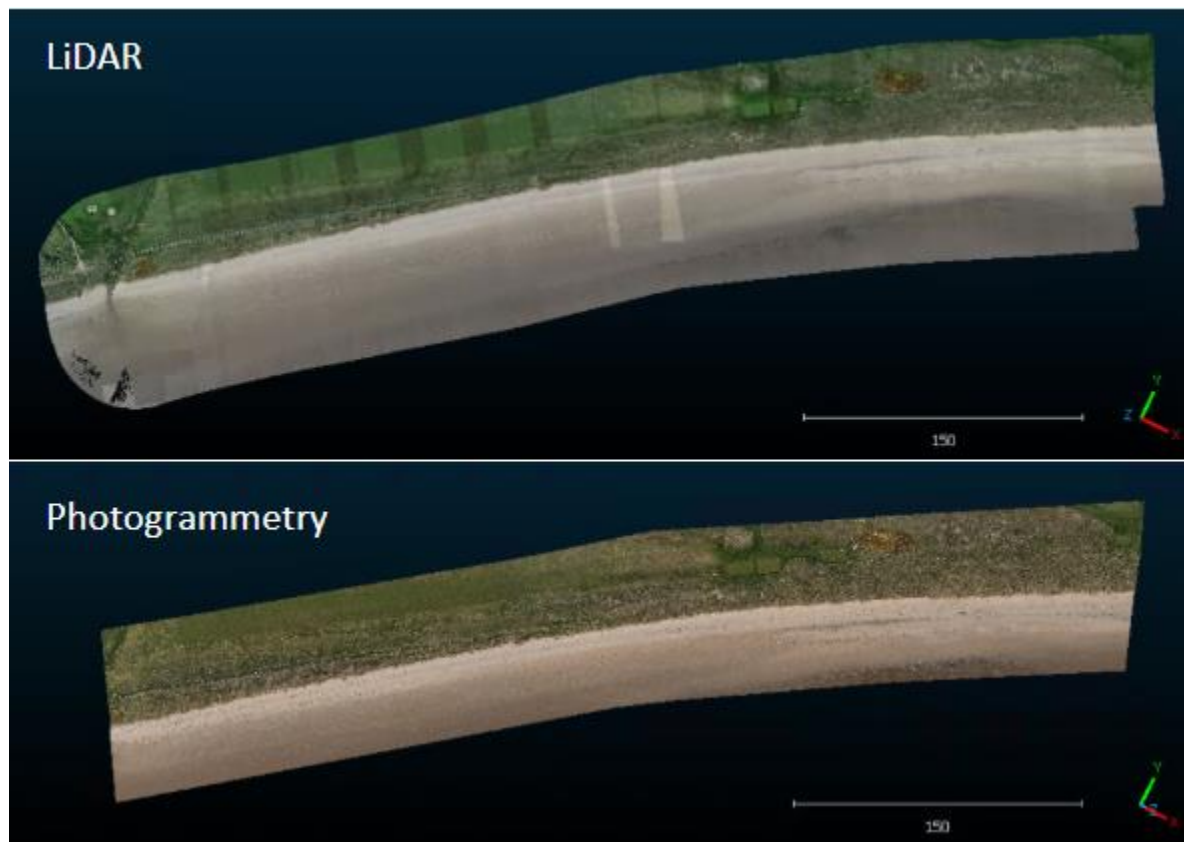
Figure 4 LiDAR and photogrammetric point clouds in CloudCompare
