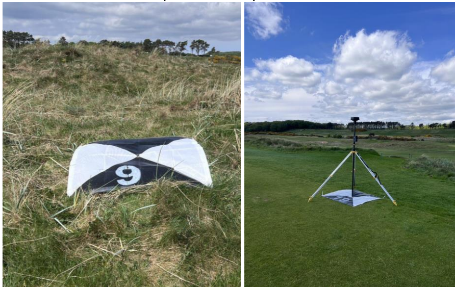
Figure 1 Ground control point and GNSS base station
