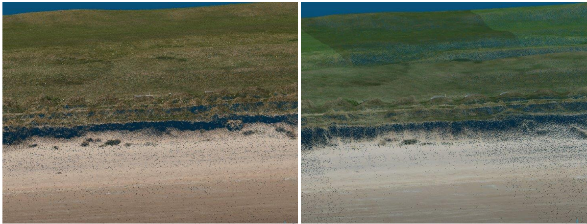
Figure 9 Point cloud of dune front showing lower density and reduced surface capture in the photogrammetry (left) dataset compared with the LiDAR (right) one
