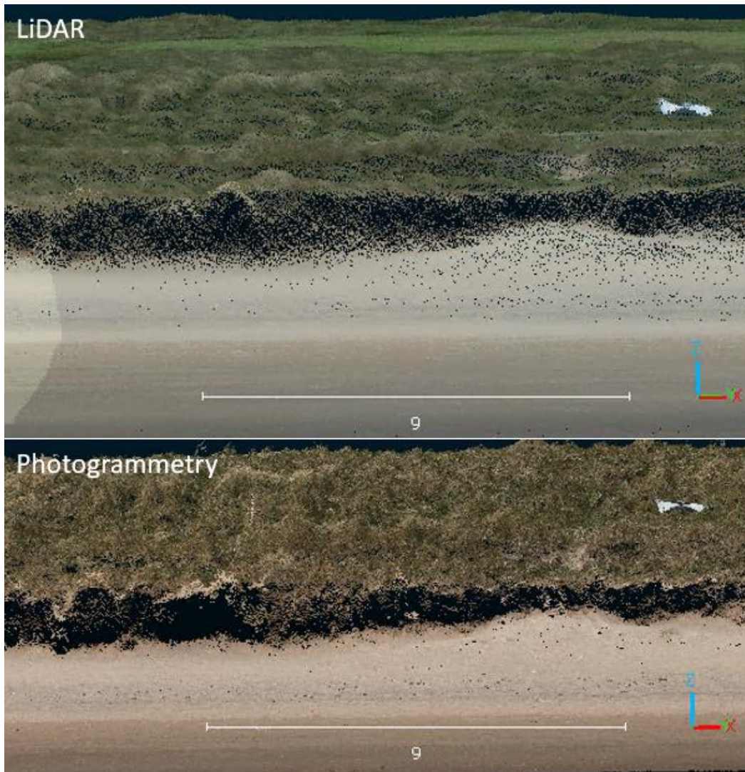
Figure 5 Point cloud of dune front showing lower density and reduced surface capture in the P1 dataset compared with the LiDAR one
