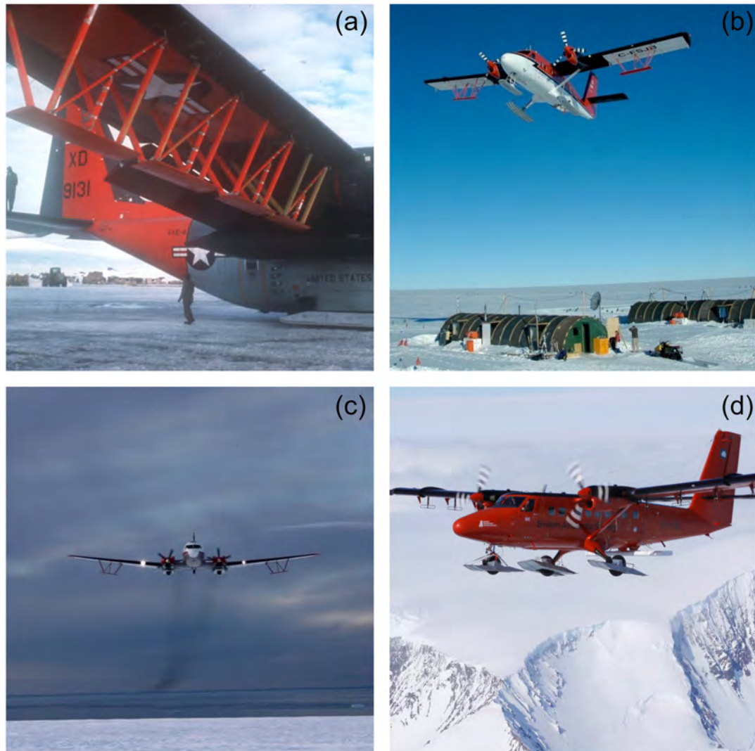
Figure 2.7: Photographs showing the evolution of airborne RES data acquisition over Antarctica. (a) LC-130 aircraft used during the 1970s RES surveys of Antarctica with the SPRI radar antennas mounted on the wings (credit: Charles Swithinbank; shared by Martin Siegert); (b) Twin-otter aircraft equipped with the University of Texas Institute for Geophysics (UTIG)'s High Capability Airborne Radar Sounder (HiCARS) system during the 2004-2005 Airborne Geophysical Survey of the Amundsen Embayment (AGASEA) survey of Thwaites Glacier (credit: Matt Fields-Johnson; shared by Duncan Young); (c) Basler aircraft during the 2008-2009 ICECAP survey using UTIG's HiCARS RES system (credit: Andrew Wright; shared by Martin Siegert); (d) Twin-otter aircraft equipped with the British Antarctic Survey (BAS)'s Polarimetric Airborne Survey INstrument (PASIN) system flying over the Antarctic Peninsula (credit: Carl Robinson).
