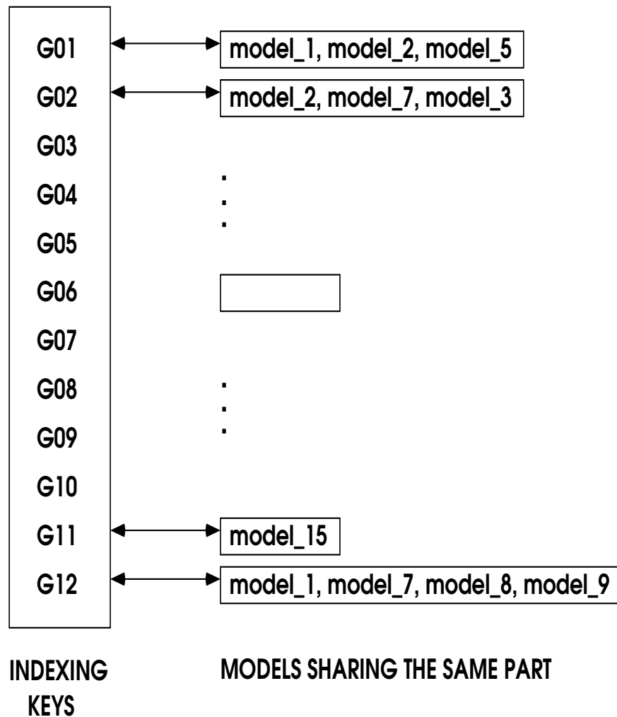
Figure 5.2: Schematic figure of the model library structure showing the geon classes as indexing keys and hypothetical models that share the pointed geons as parts.
