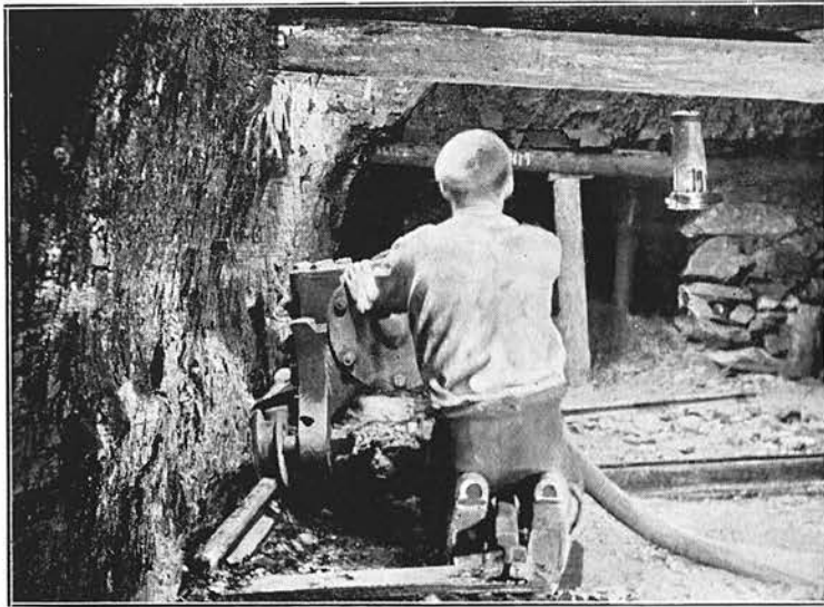
Figure 1:—Coal-cutting Machine, the Wheel having cut 5½ feet into the Coal, ready to cut forward along a Working Face, 1,920 feet long.
