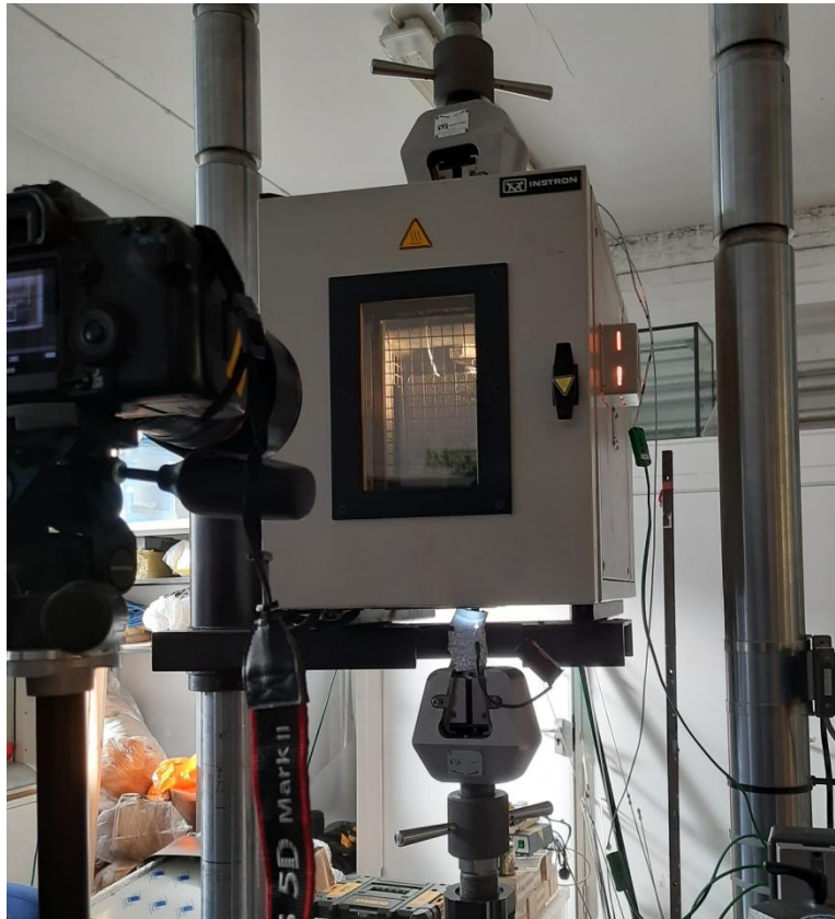
Figure 3.9. Photograph showing oven between upper and lower grips of the universal test machine, with test specimen visible through the window
