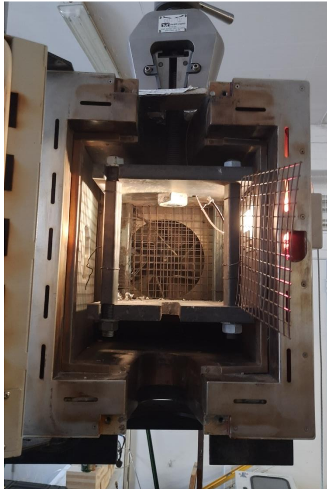
Figure 3.10. Photograph showing the steel cradle positioned inside the oven and being held from above by the upper grip of the universal test machine
