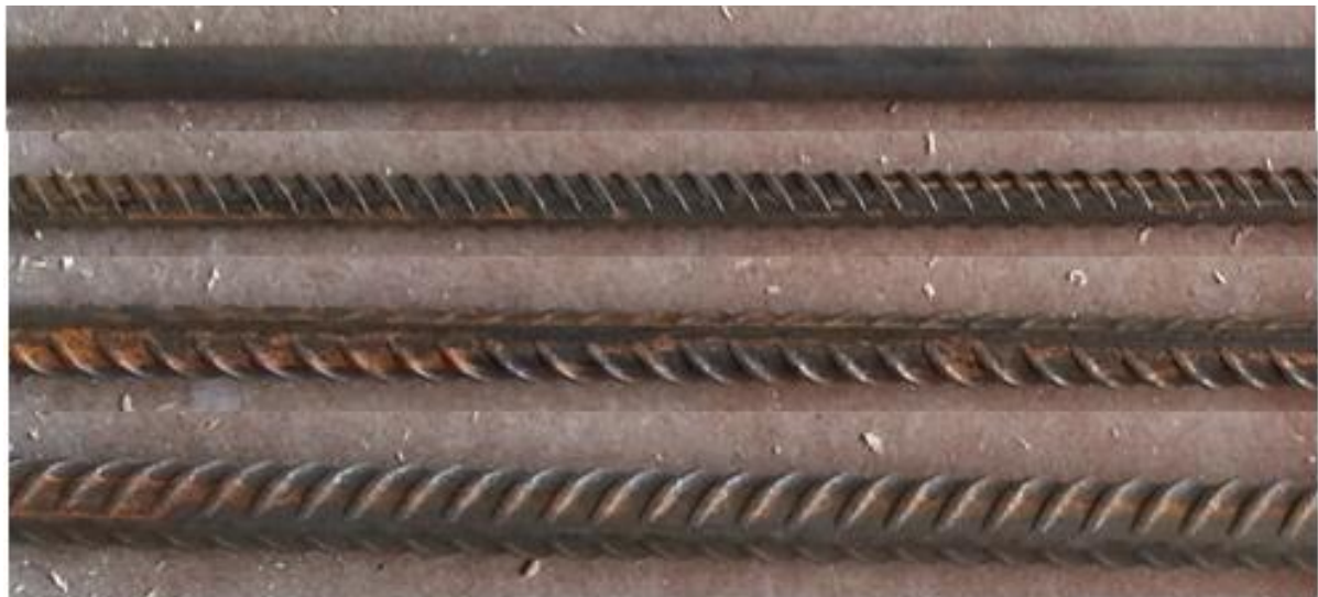
Figure 3.5. Plain bar and 8, 10 and 12mm diameter deformed bars (from top to bottom)
