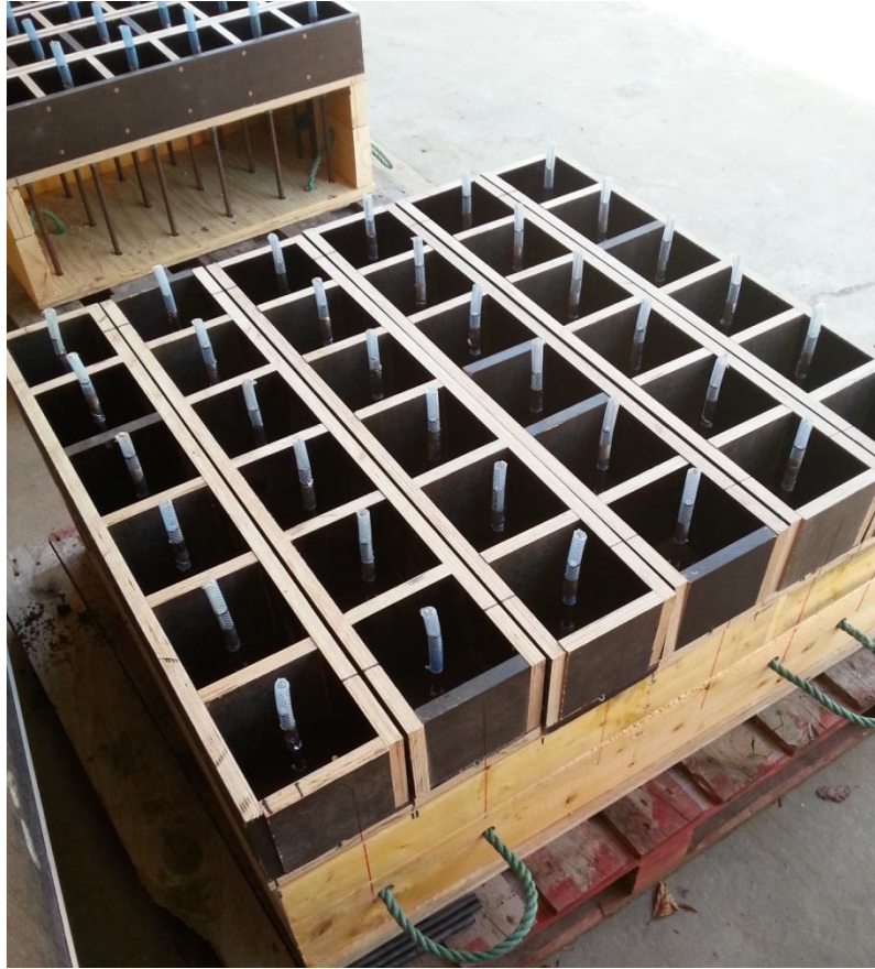
Figure 3.7. Photograph showing casting moulds for specimens with reinforcing bars in position
