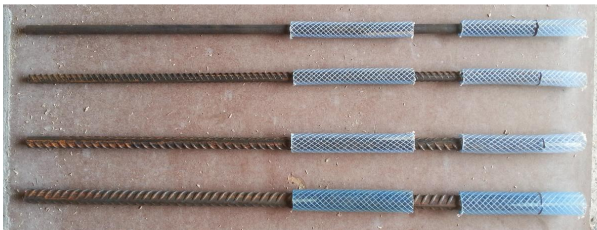
Figure 3.6. Photograph showing each bar type and diameter with hose pipe fitted in position to limit length of bonded region
