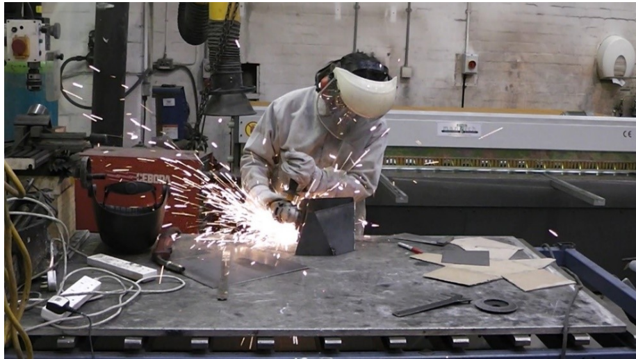
Figure 3.17. Grinding steel. Still from video
