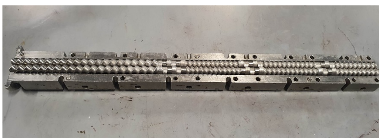
Figure 8 Interior of the extruder barrel, showing the co-rotating screw and its configuration
