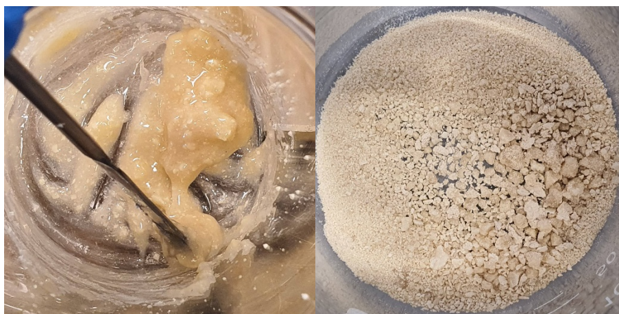
Figure 12 Colour of the product mixture for p-TPB synthesis after fed into TSE after 8 passes (Left) and colour of dried solid product (Right)
