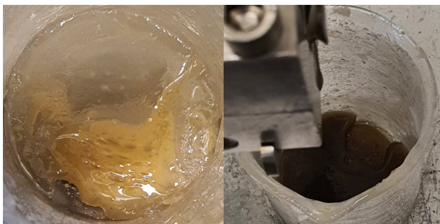
Figure 11 Colour of the product mixture for p-BA synthesis after fed into TSE after 5 passes (Left) and 8 passes (Right)
