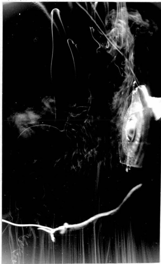
Figure 22. Nitric acid tube breaking. (Compare Figure 21.)
