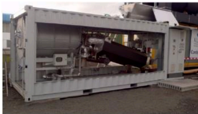
Figure 4-1. Schematic figure of PYREG pyrolysis unit.
