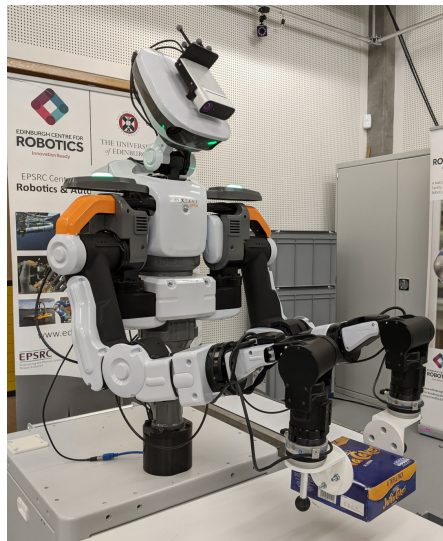
Figure 10: Experimental setup: A stationary Nextage robot detects moving objects on a conveyor using an RGB-D camera mounted on the head, picks these objects from a conveyor using custom end-effectors and places them on a table.
