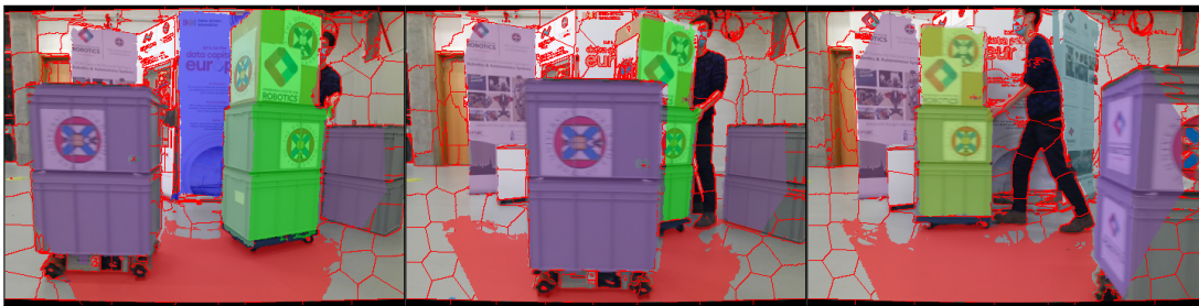
Figure 23: Hierarchical segmentation based on planes and non-planar areas. The planes are extracted from the depth map and the non-planar areas are represented by a set of super-pixels.
