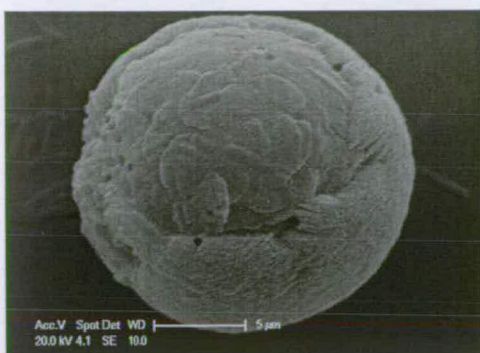
Figure 6.4ai. SEM image of EPS-free cell experiment at 48 hrs (showing detail of spherical precipitate).
