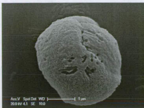
Figure 6.4aii. SEM image of EPS-free cell experiment at 48 hrs (showing surface detail of precipitate).
