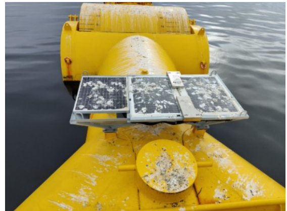
Fig.7 Soiled Panels during the deployment
