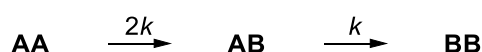
Scheme 7.1: A sequence of two consecutive unimolecular reactions where equivalent and independent reactive sites A react to form B.
