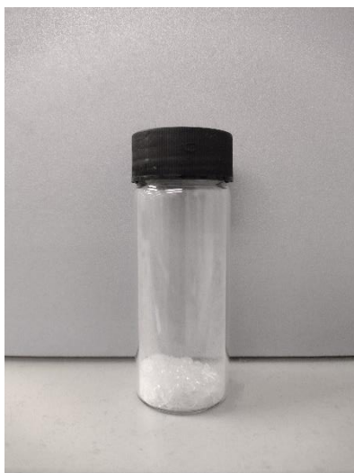
Figure 5.1: Powdered glass prepared from a Fisher Scientific borosilicate glass Pasteur pipette.
