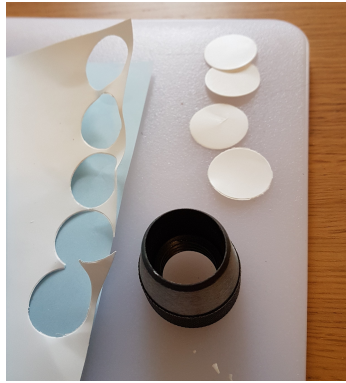
Figure 2.6: Membrane cutting process using 13 mm diameter leather punch. The membrane sheet was laid down on a cutting board and the punch was then used to carve out each membrane individually. Although the process was not significantly more time consuming than laser cutting, the percentage of usable membranes was reduced due to mistakes and defects in the sheet, which could easily bend and be damaged by touch during the process. Each membrane was then carefully inspected before being placed into the devices for assembly.
