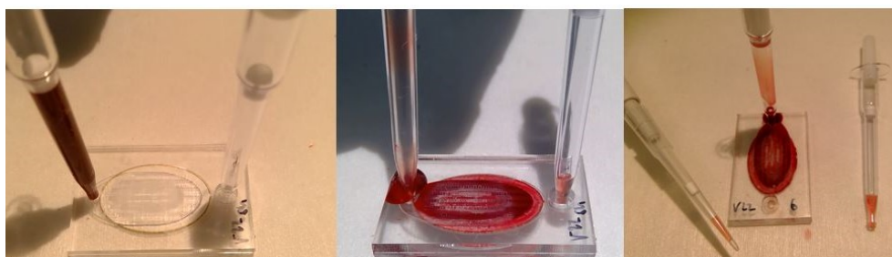
Figure 4.10: Testing process of the “double Minivette” setup, where a second Minivette was used to collect the plasma from the output. Left to right: the blood is pushed inside the Minivette. The second Minivette starts absorbing the output plasma, but fails to complete the collection process, which was finished using a pipette.
