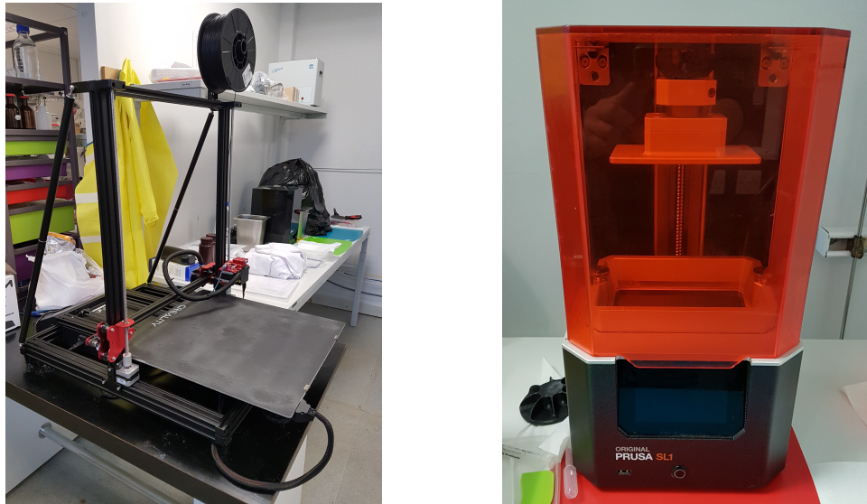
Figure 2.4: Example of an affordable type of FDM (left) and MSLA (right) 3D printer. In the FDM format, a filament is melted and extruded out of a hot nozzle to construct the 3D printer object, while in the MSLA printer liquid resins is polymerised through UV light exposure to form each of the object's layers.
