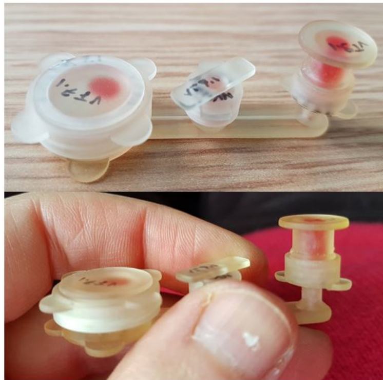
Figure 8.13: Top: example of all air-tight enclosure, needle valve and actuator integrated into a single device and tested with water and red food colouring. Bottom: view of the same device from a different angle.
