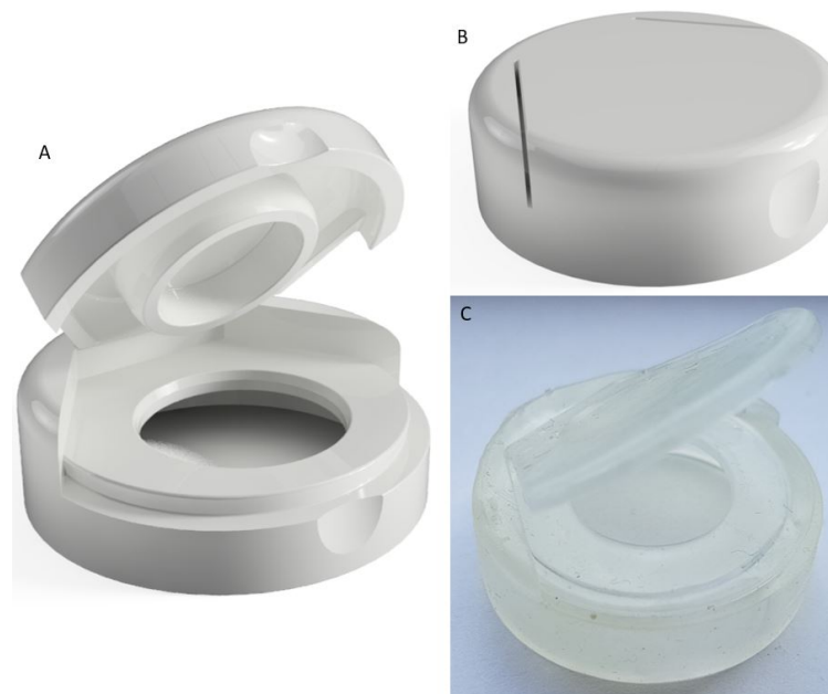
Figure 8.1: Design and 3D printed object of the first enclosure attempted. A) Rendered version of the enclosure. The top and bottom parts are connected through a hinge and the edges connect through a snap-fit mechanism. B) Closed version of the enclosure, with the snap-fit mechanism engaged. C) Object 3D printed using flexible resin.
