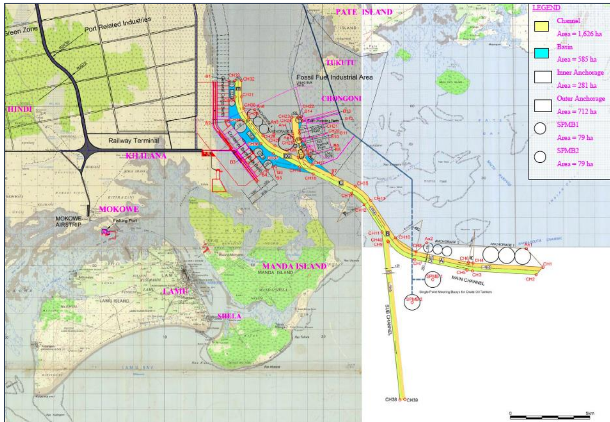
Figure 12: Lamu port design, source: Japan Port Consultants (2011)
