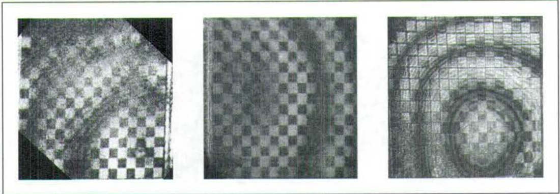
Figure 3.8: 256^2 SLMs displaying a 16^2 checker pattern; note the fringing and contrast reversal caused by varying cell gap.
