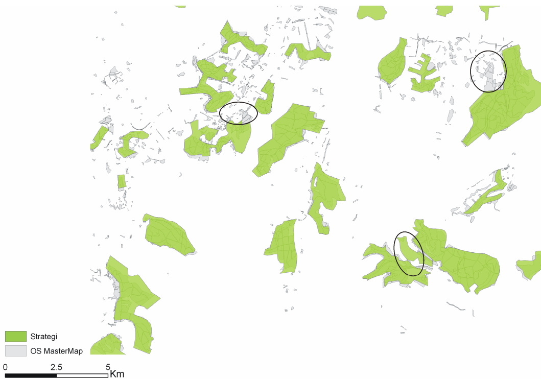
Figure 13: Significant differences between the Strategi and the source data because of displacement, classification error, and change of landuse between updates (Mapping is Ordnance Survey ©Crown Copyright. All rights reserved)
