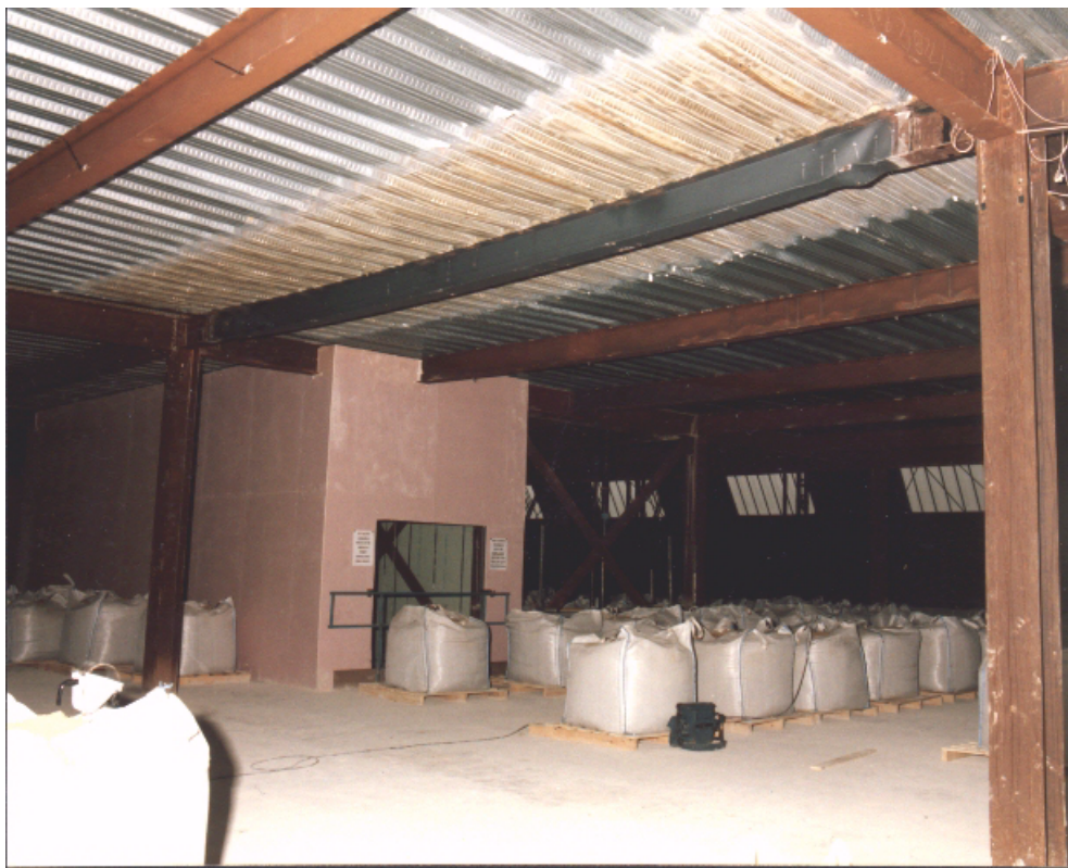
Figure 4.3: British Steel Test 1: Restrained beam test
