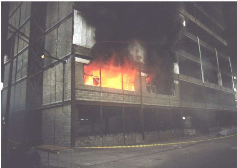
Figure 4.7: Compartment fire in progress in British Steel Test 4: Office demonstration test
