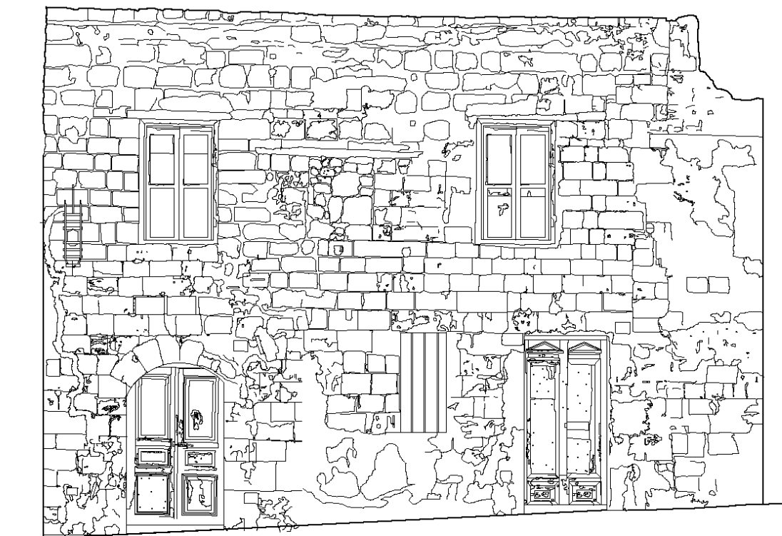
Figure 81: Documentation and mapping of the main facade
