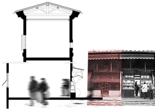
[1] Section across the East side of the Ponte Vecchio, with its characteristic wooden shutters known as 'argani' (winches).
