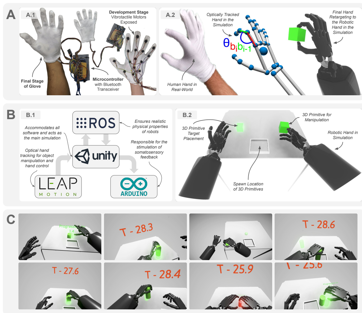
Figure 3.2: Simulation, hand-control and interface overview. The figure depicts the overall apparatus, including the simulation overview, the employed hand-control procedure and snapshots of the simulation. Figure A.1: The development of the custom-built somatosensory capable haptic glove. Early and final development stages are depicted. Figure A.2: The employed hand-retargeting approach, tracking the hand of the human participants in the real world (either with or without the glove), the corresponding tracked hand in the simulation and the final hand-retargeting to the robotic hand. Figure B.1: The simulation overview with all software used, arrows indicate information and data flow. Figure B.2: The overview of the motor task in the simulation with the hand-re-targeting approach in full working order. Figure C: Participant recordings in the simulation performing the different motor task experiments across varying sensory interfaces.
