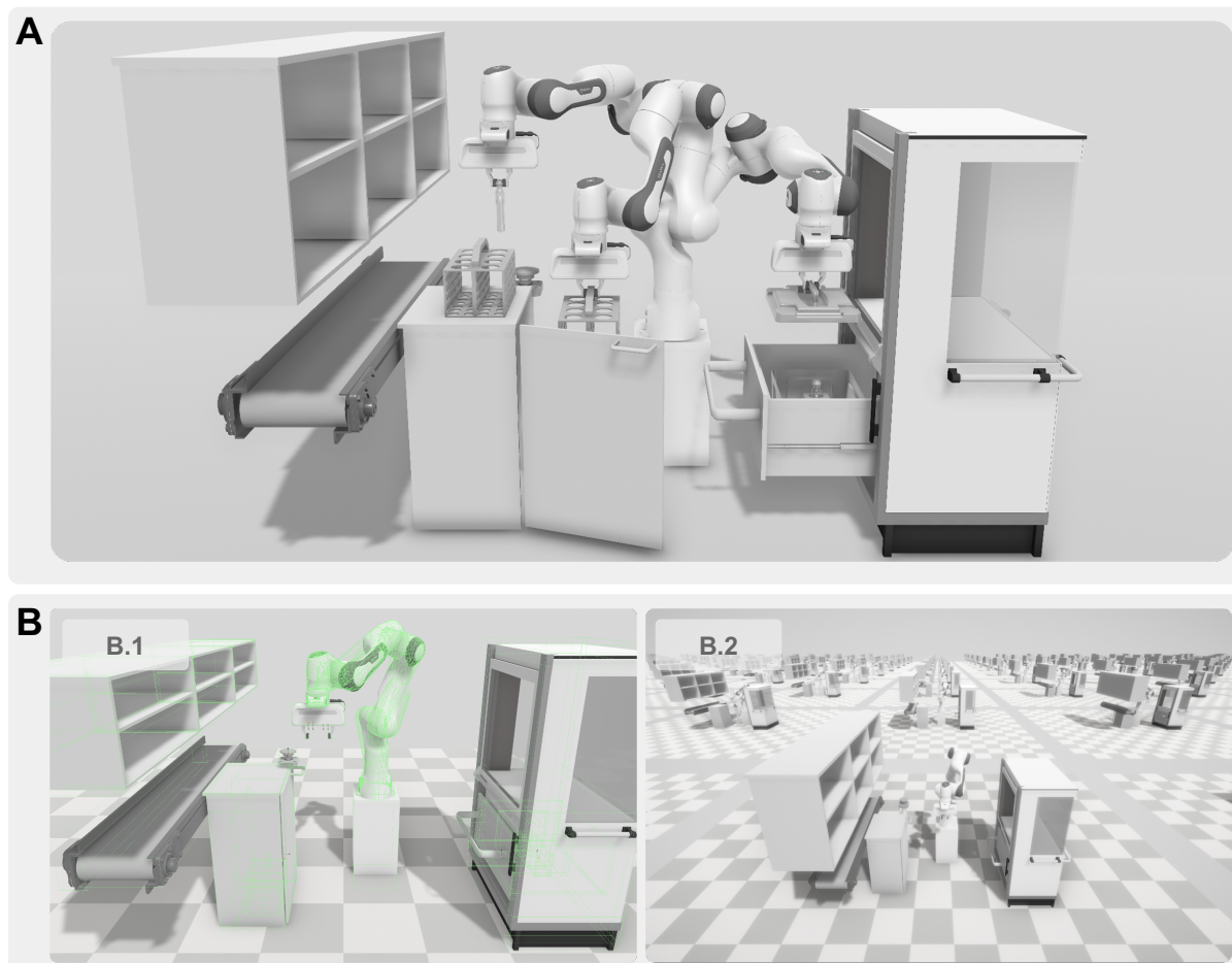
Figure 5.3: The simulation setup of ROMAN. The figure depicts the simulation, showcasing ROMAN and in particular the task in closer detail. Figure A: The simulation environment of ROMAN visualised with distinct key snapshots of its operation and in particular all phases concerned with picking . The figure serves as a brief visual overview of the task. Figure B.1: The rigid bodies and colliders highlighted in green, of both the Franka Emika Robot, served as the main robot to test ROMAN on, including the surrounding environment. These colliders, alongside the physics configurations, presented themselves as a promising validation environment entailing realistic physics-based interactions. Figure B.2: The illustration of the parallelism of training ROMAN, which allowed for a notably reduced real wall-clock training times by virtue of utilising concurrent instances of the learning scene.
