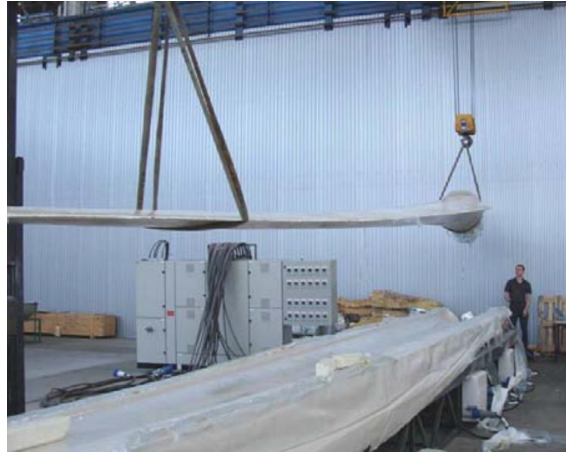
Figure 2.3: A 12.6 m long recyclable wind turbine blade made by ÉireComposites from CBT ® thermoplastic resin. Half of the heated concrete mould used to produce the blade is visible at the bottom. Reproduced from [32].
