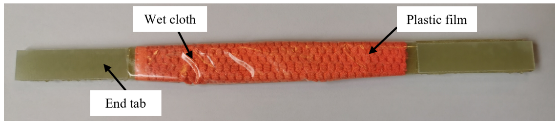
Figure 5.1: Aged coupons were kept wet during testing by covering with a saturated cloth and plastic wrap.
