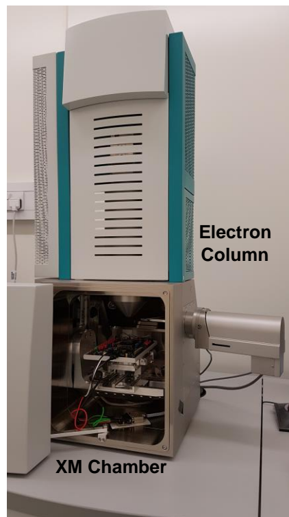
Figure 3.7. Tescan Vega 3 SEM showing electron beam column, XM chamber and SPAD image sensor with operational circuitry.
