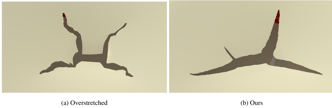
Figure 4.6: Extreme over-stretching produced when cutting a thin shell by the original phase field method (Fig. 4.6a) and our proposed method (Fig. 4.6b).
