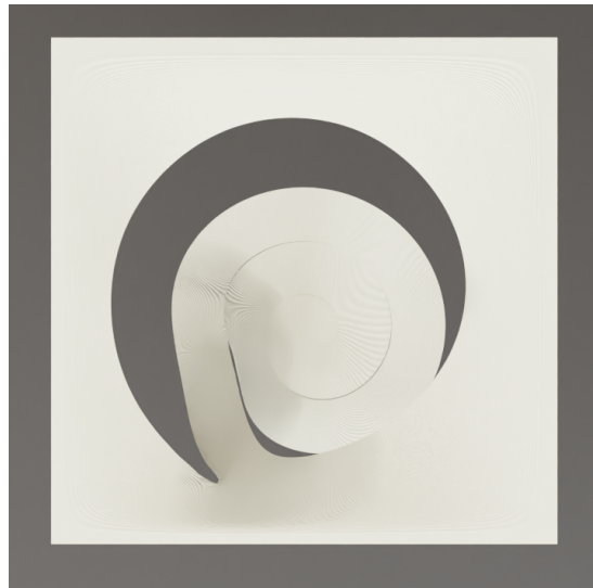
Figure 4.21: A sheet is pre-cut with an Archimedean Spiral curve. Our MLS formulation enables exact cutting with complex crack geometry.
