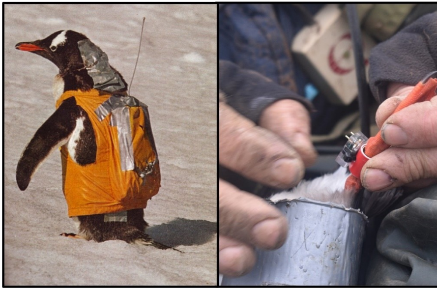
Figure 20. Left: A radio backpack fixed on a Gentoo penguin in 1972 (source: National Geographic). Right: A geolocator attached to an Atlantic Puffin (Grímsey, 14.06.2024).
