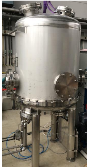
Figure 31 – The assembled TOPOFLAME rig before a test takes place, the inner volumetric capacity of the chamber is 1000 L. The total height of the chamber is 2.6 m.
