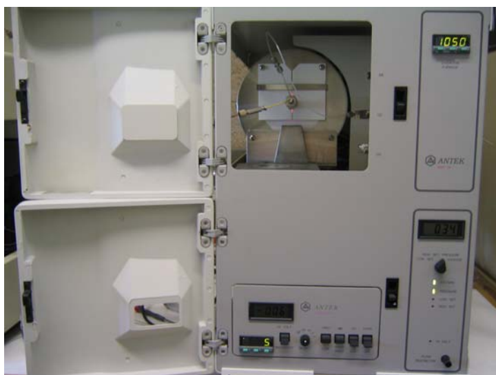
Figure 2.4: The ANTEK 8060-M nitrogen specific HPLC detector.
