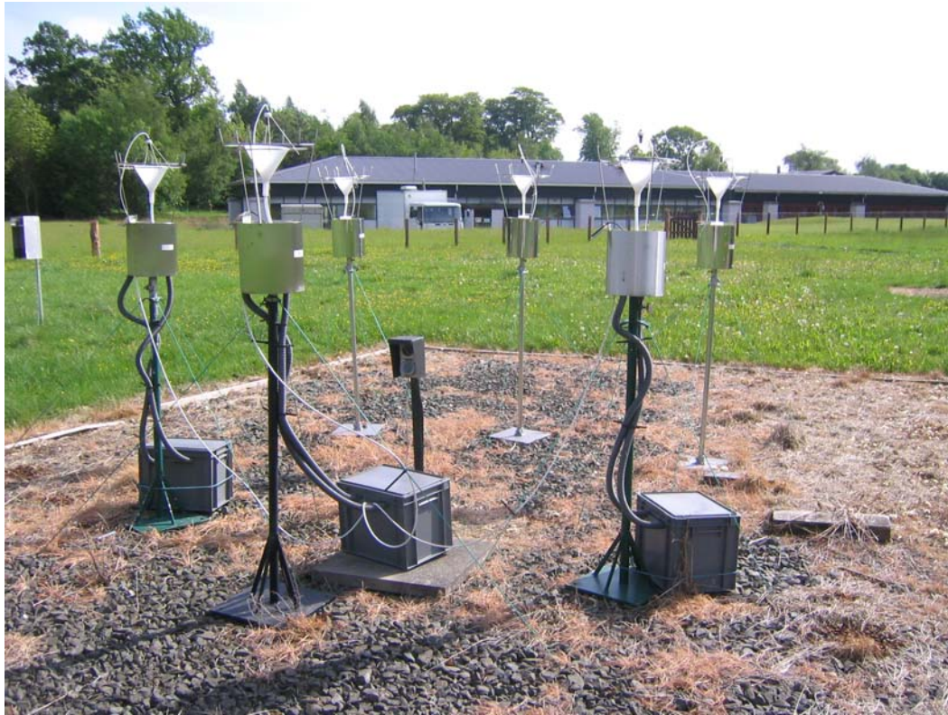
Figure 3.1: Standard rain collectors and flushing rain collectors at the CEH, Edinburgh.
