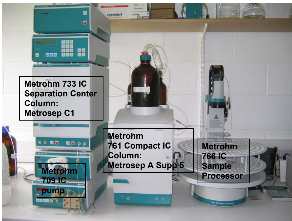
Figure 2.1: The ion chromatography (IC) equipment: a Metrohm 766 IC Sample Processor connected in parallel to a Metrohm 761 Compact IC equipped with a Metrosep A Supp 5 column (for anions analysis) and a Metrohm 733 IC Separation Center equipped with a Metrosep C1 column (for cations analysis).
