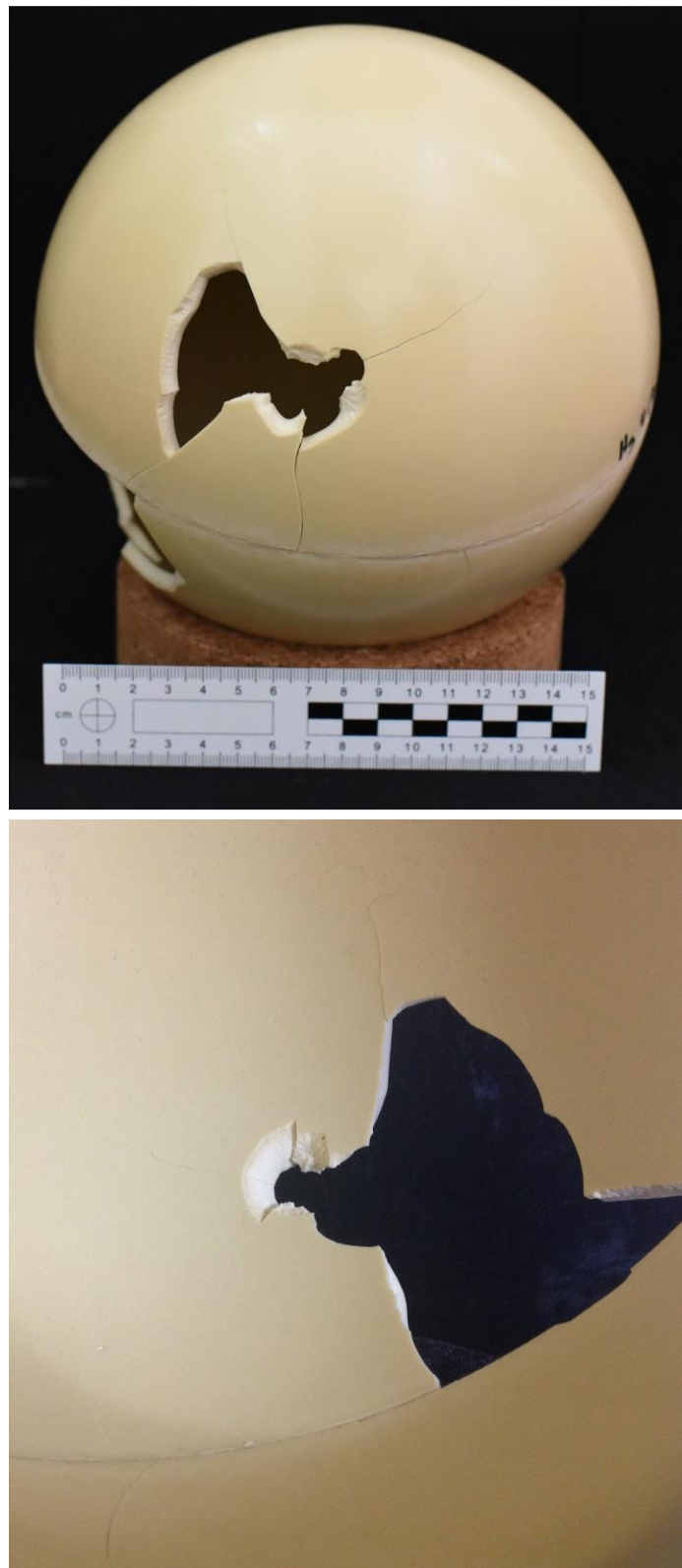
Figure 6.1. Sample Hg 4 (9 mm), where bevelling is present on both the external (top) and internal (bottom) table of the entrance defect due to a tangential strike.
