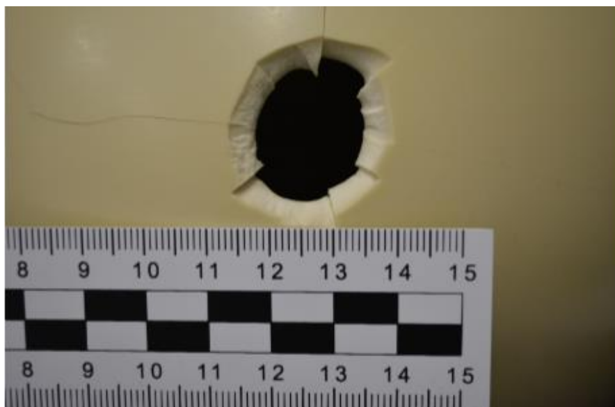
Figure 3.16. Exit defect with external bevelling (sample Ri4).
