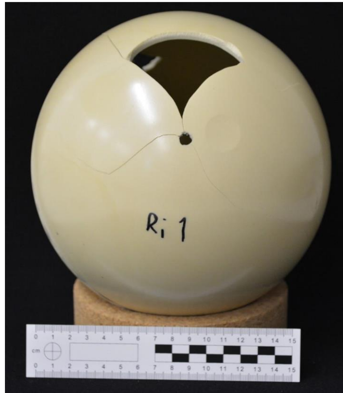
Figure 4.10. Sample where reconstructing the entrance defect does not affect the diameter of the entrance itself (Sample Ri 1).
