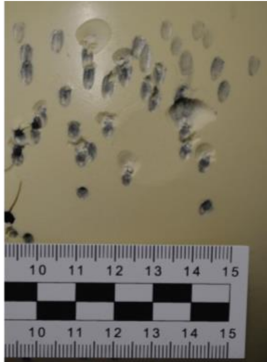
Figure 3.17. Residue at impact sites (sample Sh1).
