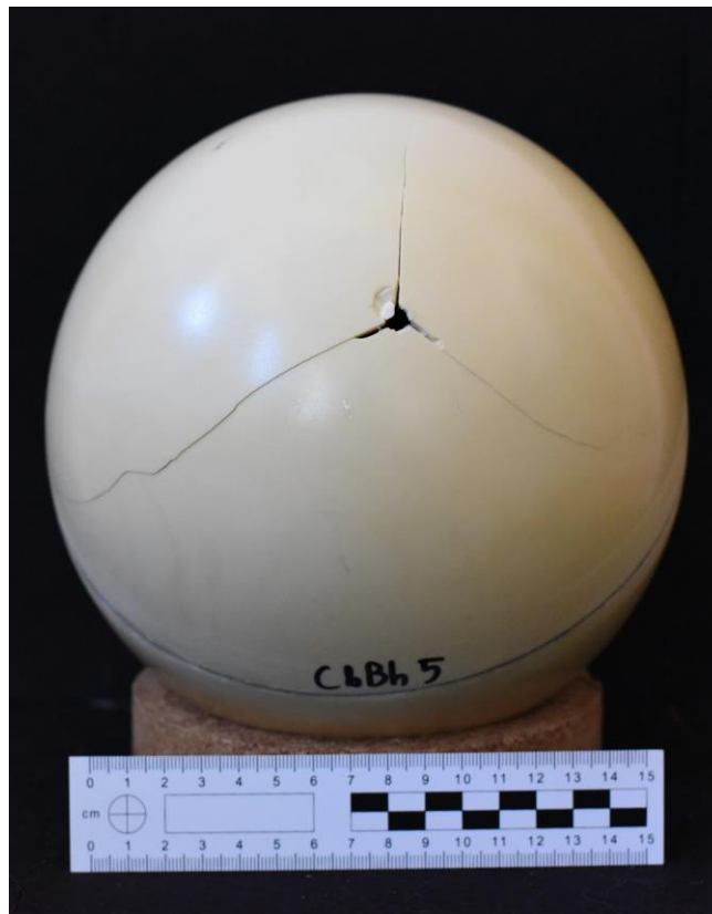
Figure 4.45. Entrance defect of fixed broadhead sample (CbBh 5) where the fracture pattern reflects the arrangement of the three-blade tip.
