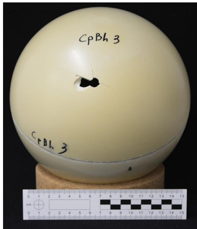
Figure 4.29. Keyhole defect at the entrance site (sample CpBh 3).
