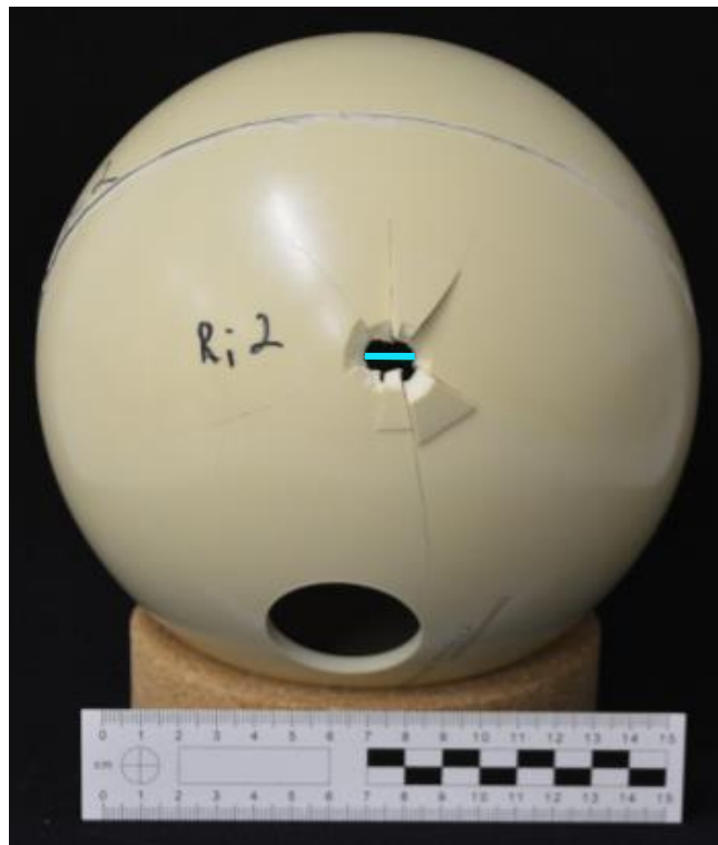
Figure 3.21. Reconstructed exit (sample Ri2). Blue line indicates maximum exit diameter.
