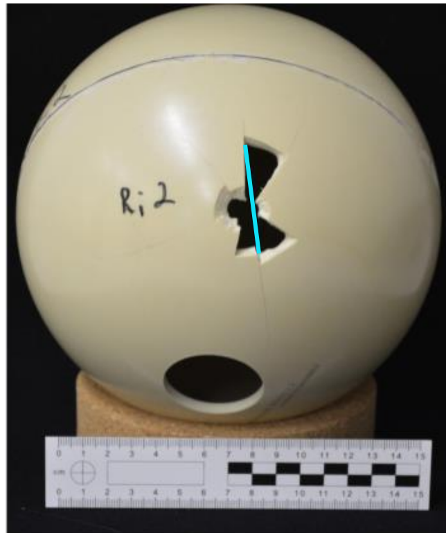
Figure 3.20. Exit without reconstruction (sample Ri2). Blue line indicates maximum diameter.
