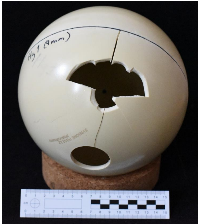
Figure 3.9. Exit defect of sample Hg 1 (9 mm) after reconstruction using recovered dislodged fragments. Reconstruction incomplete due to missing fragments.
