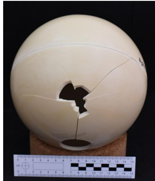
Figure 4.6. Reconstruction of exit site (sample Hg 2 (9 mm)), which greatly affects the diameter of the defect. Top: exit defect without reconstruction; Bottom: exit site with reconstruction.
