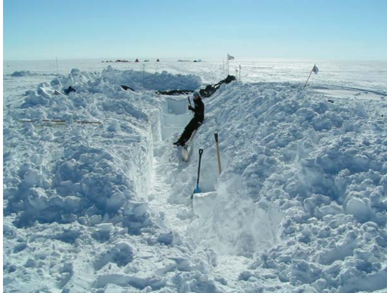
Figure 57: The ~7 m trench looking west, i.e. the far end (furthest from the camera) is nearest to T5. The far end is divided into three 'pits' ~2 m deep. The end closest to the camera is ~90 cm deep.
