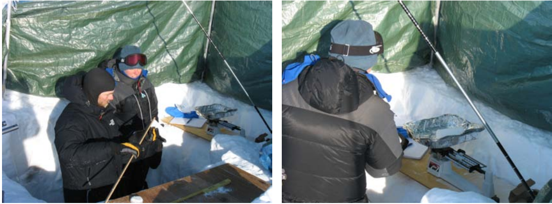
Figure 25: Logging the core, measuring cylindrical sections, and then weighing them on a triple beam balance, protected from the wind by a tarpaulin shelter.
