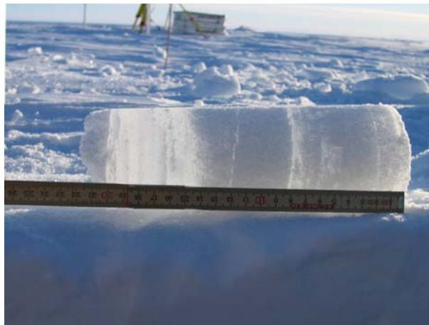
Figure 24: Section of core retrieved from drilling showing one clear large ice layer, and other ice features.
