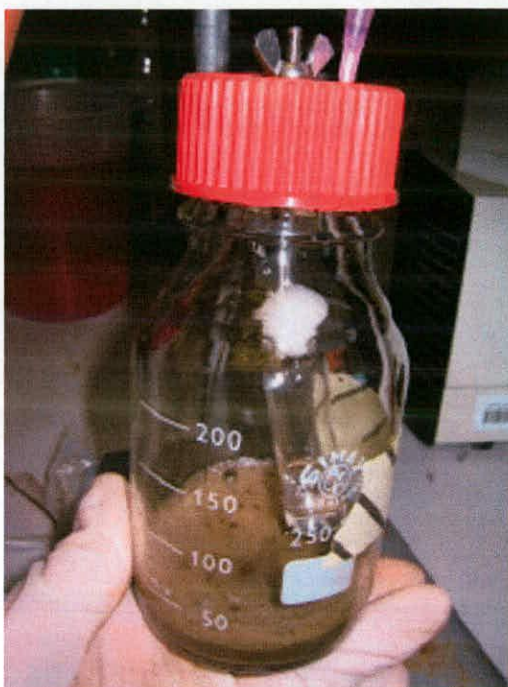
Plate 7.1 Soil respirometer under preparation. The bubbles on the surface of the soil slurry are a result of the vacuum being applied via the needle piercing the Teflon liner through a hole in the cap. Also visible are the stainless steel rod and crocodile clip
