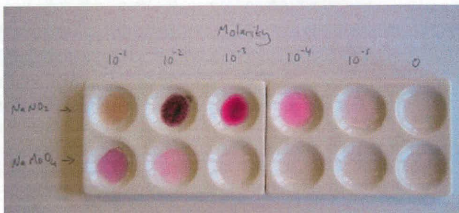
Plate 6.2 Nitrite test on various dilutions of \text{NaNO}_2 and \text{NaMoO}_4 to show interference from molybdate
