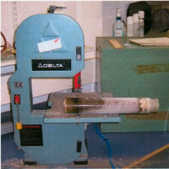
Plate 8.3 Sectioning frozen columns
