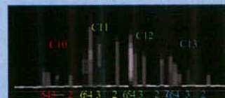
Figure 3. Typical GC of fresh LAB cable oil. Annotated with alkyl chain length and position of phenyl group.
