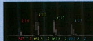
Figure 4. GC of LAB cable oil exposed to nitrate as a TEA (after 13 weeks).
