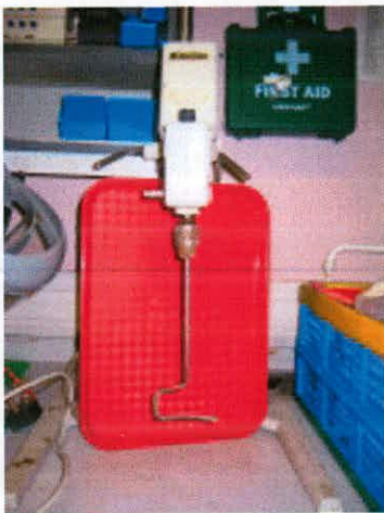
Plate 5.1 Apparatus used to mix soil and LAB
