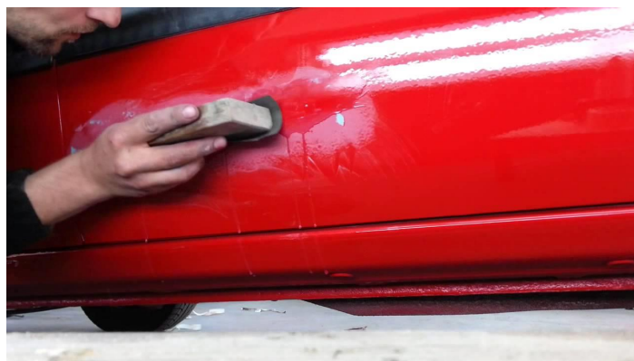
Figure 2.5: This figure shows a man trying to even a run on his car paint [41].
