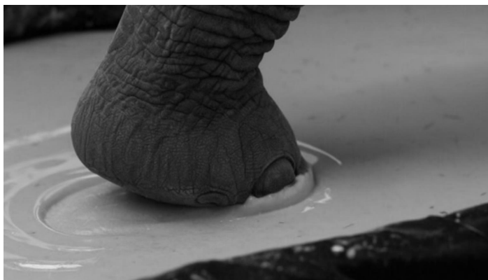
Figure 2.7: Here we show elephant running on cornstarch and water mixture (often called oobleck) which exhibits discontinuous shear thickening behaviour [23].
