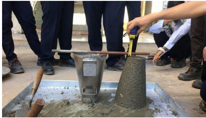
Figure 2.3: Here we show a man performing concrete slump tests, which is a measurement of concrete workability and fluidity [30].
