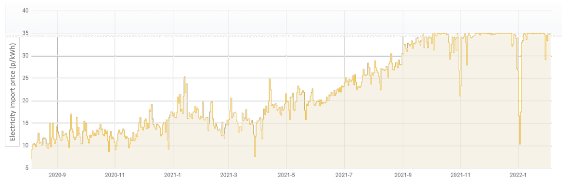
Figure 4.11: Average Agile import prices in North Scotland for the last 18 months which shows the effect of gas supply scarcity starting in October 2021 where the price is capped at 35p/kWh - data from [8].
