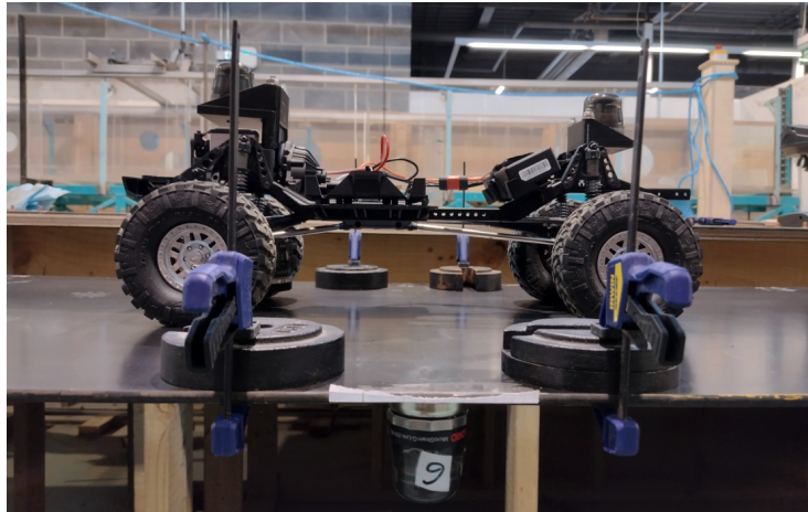
Figure 7.2.2: Vehicle used for laboratory testing at University College Dublin, showing accelerometers mounted to the vehicle and underside of bridge deck and added masses clamped to the bridge deck.
