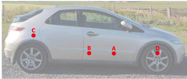
Figure 4.3.1: Vehicle used for fieldwork, showing sensor locations in phase 1.
