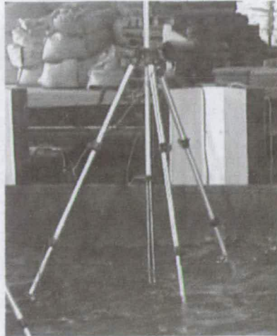
Figure 10: Twin wire resistance wave gauge mounted on a tripod
