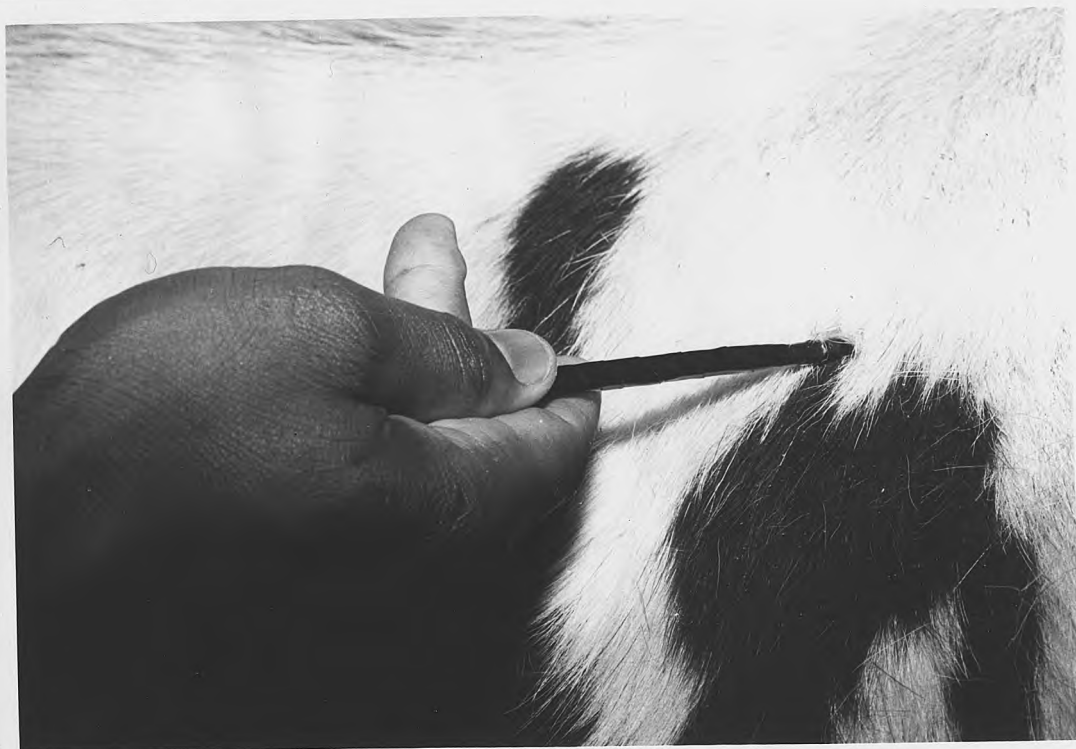
Plate 4. Thermocouple - Measurement of Skin Temperature.
