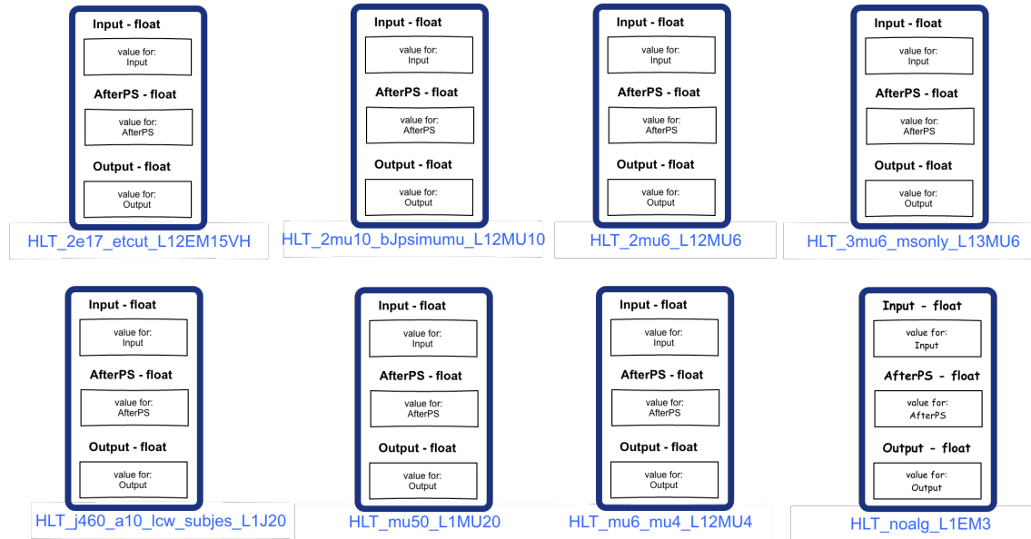
Figure 4.3: Illustration of the class used by TRP to broadcast monitoring information during Run 3. Each instance of the class contains the values for a single trigger rate. Multiple instances of the class are being published (one for each trigger rate). Using this approach, the trigger rates can be selected by name in the new Grafana dashboard.
