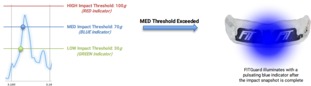
Figure 2.2: Example impact snapshot and threshold levels that illuminate LED within the sensor strip (image courtesy of FIT (2014), unpublished).
