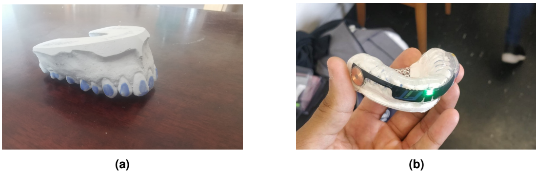
Figure 2.3: (a) Example mouth-mould for a player and (b) mouth-mould with instrumented mouthguard moulded around it.
