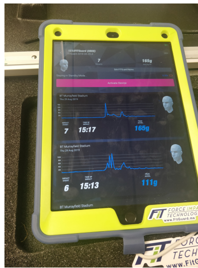
Figure 2.8: Tablet device connected with instrumented mouthguard, showcasing the downloaded impacts from a session
